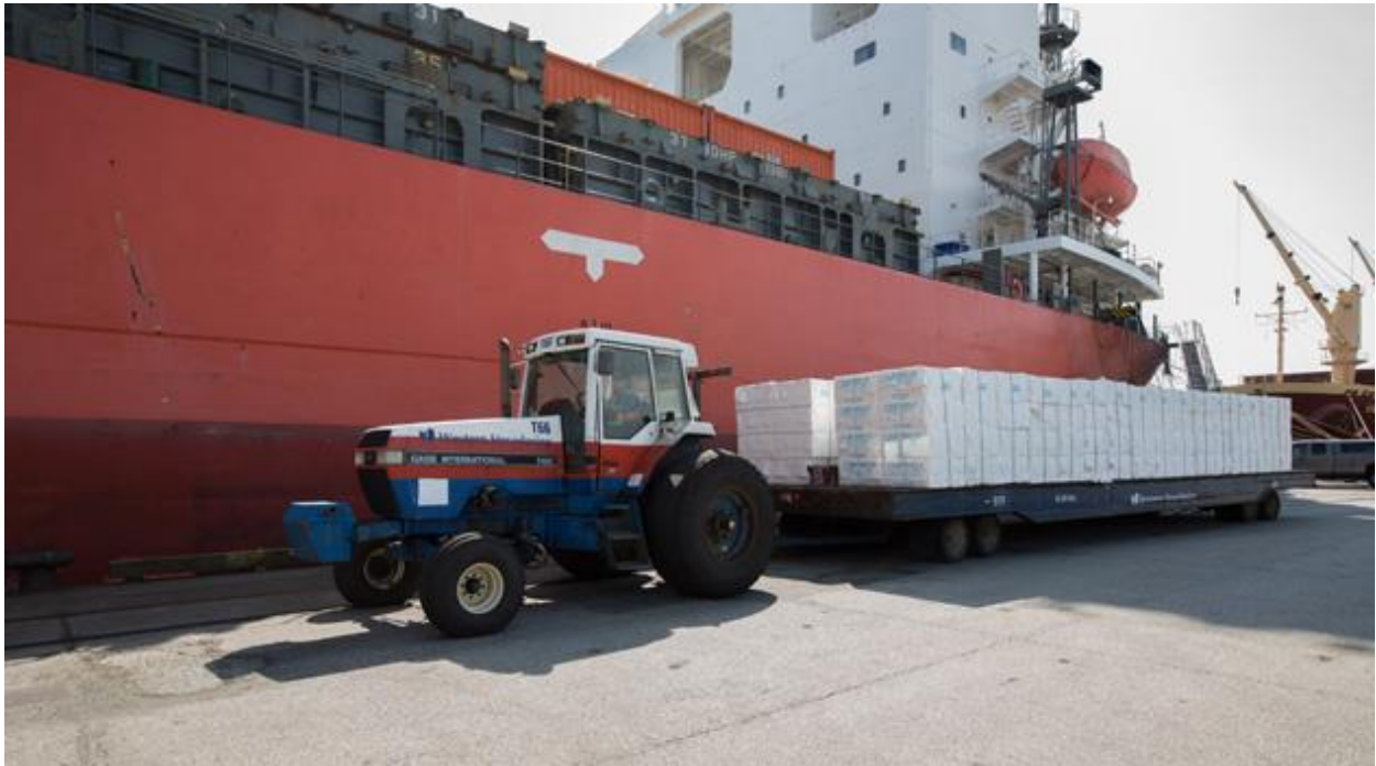
The typical cart equipment required to deliver bales alongside the vessel for loading or to receive the bales as they are unloaded from the vessel.
